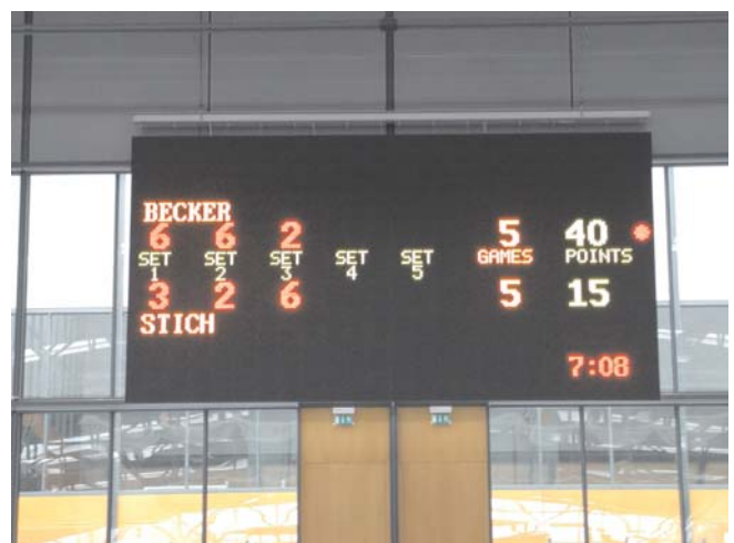
Example: 11 m 2 with 32 x 8 Characters at 20 cm heighth From this size the three coloured system RG96 can be used without any restrictions.
